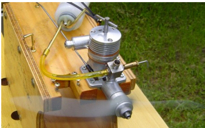
The 1.5cc will happily pull 10,000 RPM with the correct prop.
