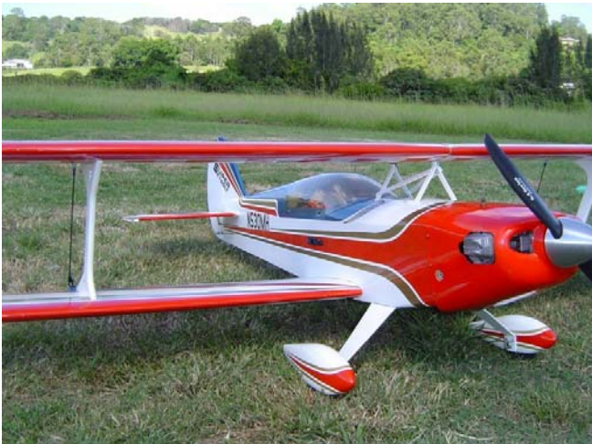
The Skybolt weighs in at about 8.5lb and the OS 91 provides ample power.
